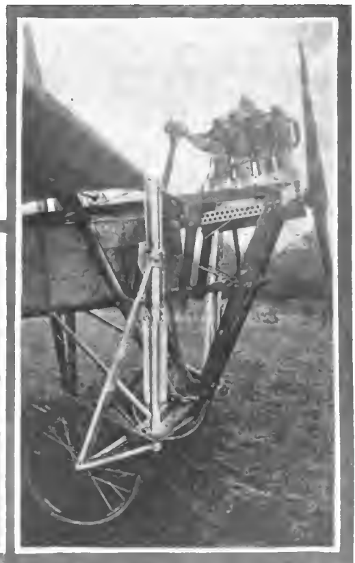
Cellier Monoplane, Showing Panhard Engine
